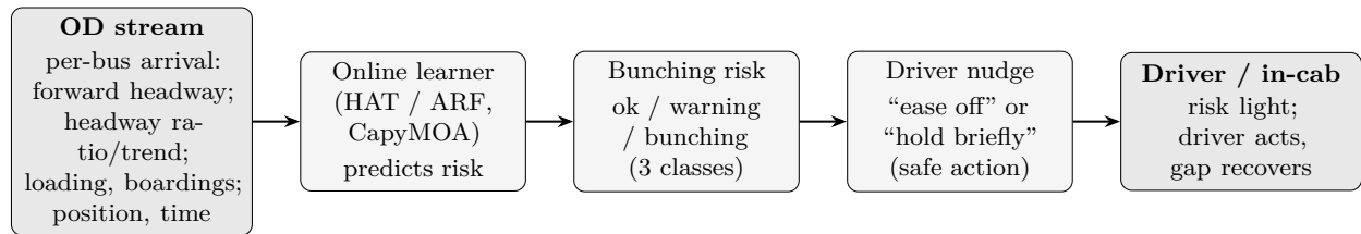
Figure 2: Runtime flow of the driver-nudge system. The online learner ingests the per-bus features of each arrival, predicts the next-window bunching risk, and a warning or bunching class triggers a safe nudge that the driver can act on so the impending bunching is averted.
